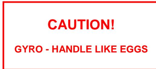
The gyro and supporting frames or gimbals run on very delicate bearings which are able to absorb the normal range of aircraft flight manoeuvres and landing loads when correctly installed and operating. However, gyro instruments will soon give increasingly erroneous readings after having suffered jarring or shocks resulting from heavy landings or rough handling during installation or bumps and shocks inflicted while being moved from the store to the aircraft or during shipping.
