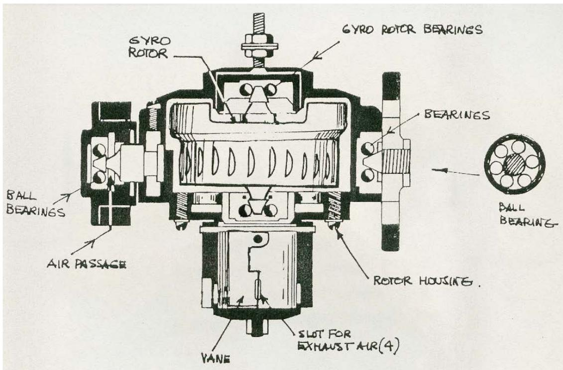
A typical classic air-driven vertical spin axis gyroscope (artificial horizon) design showing typical bearing arrangement and low bearing contact area which makes the bearings susceptible to any shock damage.
