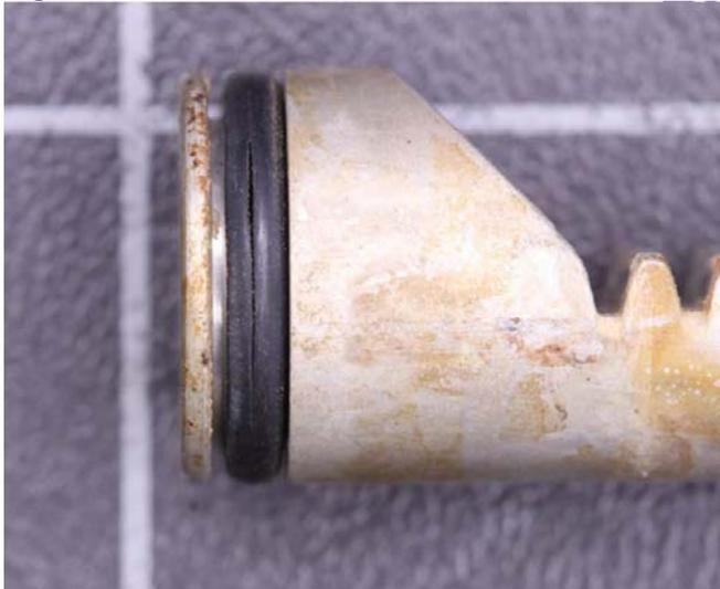
**Failed fuel selector spool seal. All four seals in both valves showed similar deterioration. Source ATSB**
