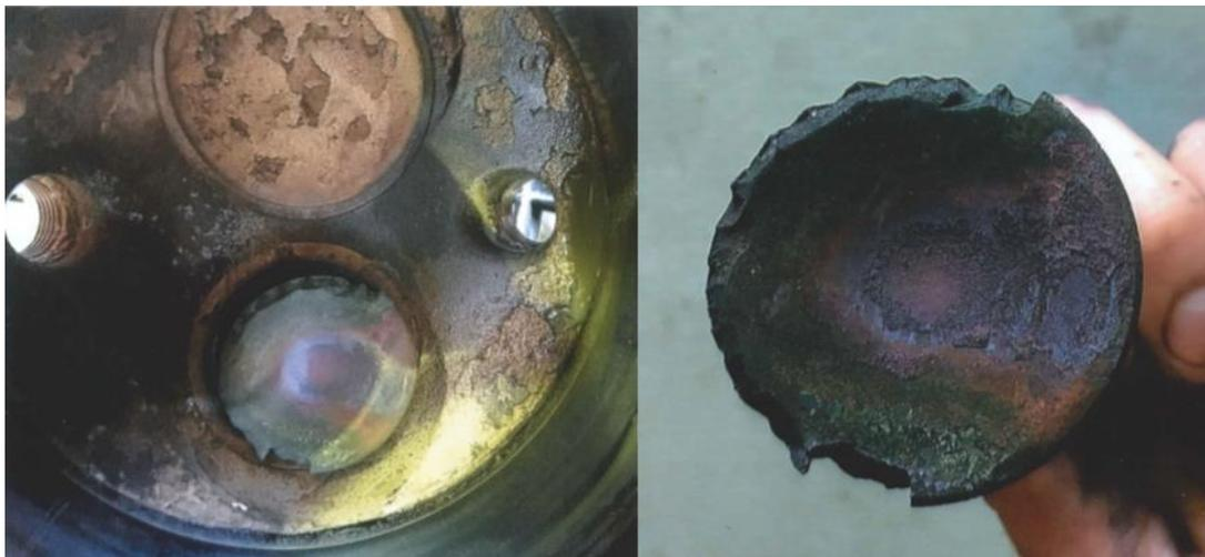
Images of Exhaust Valve Seat Degradation and Valve Chipping
