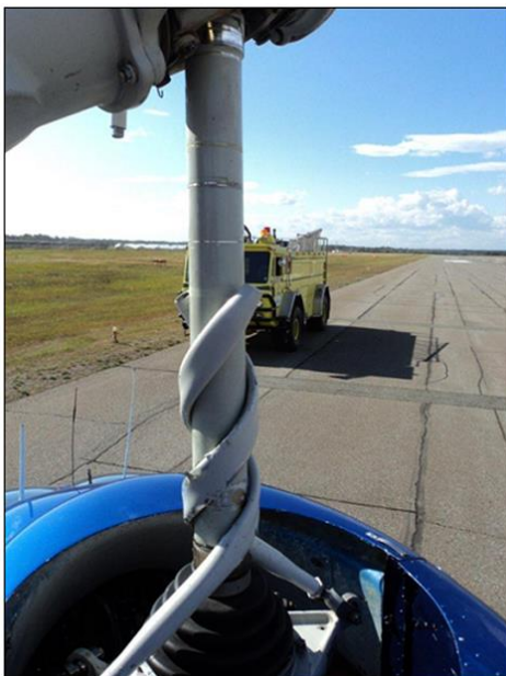
Fig 1. - Main rotor mast to rotor head separation failure. Accompanying text is a summary based on TSB Aviation Investigation Report A11C0152.
