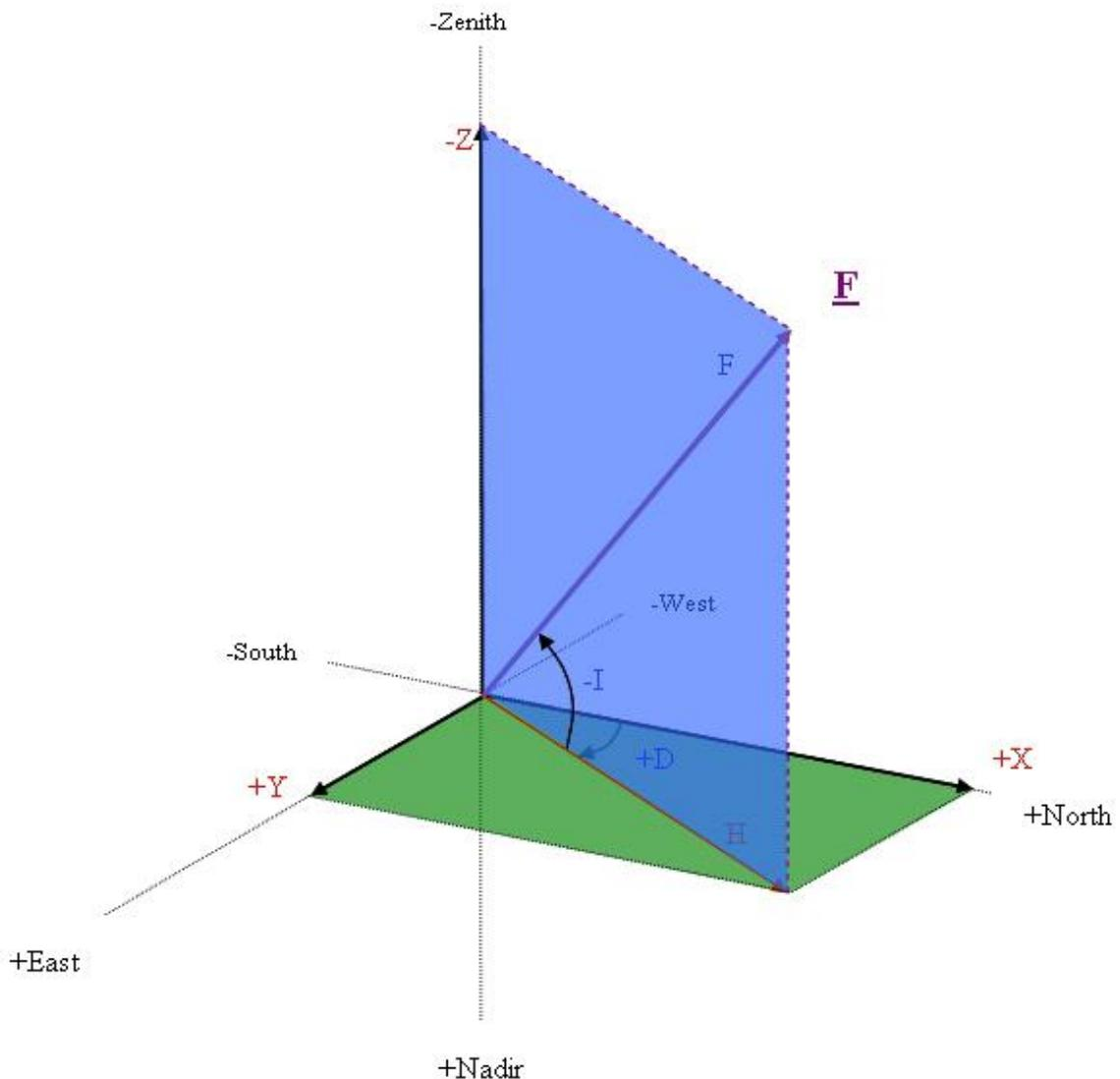
**Figure 1 - Components of magnetic vector (source Geoscience Australia)**
