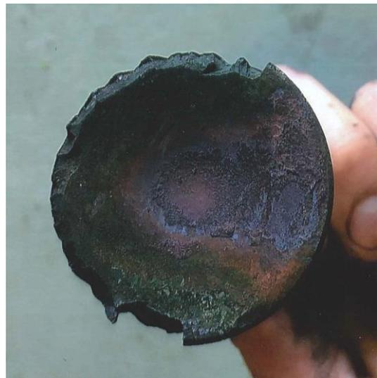
Images of Exhaust Valve Seat Degradation and Valve Chipping
