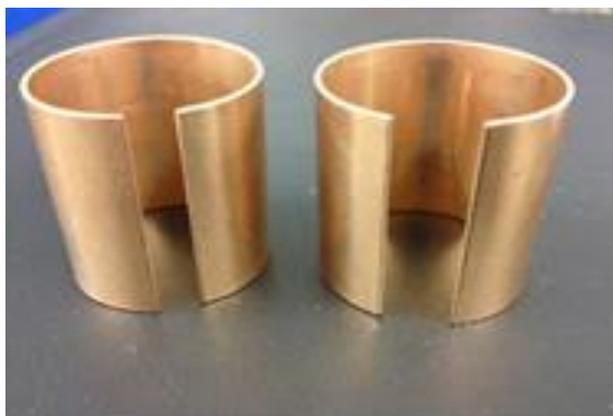
Figure 1 - The bush on the right is a Connecting Rod Small End Bush P/N LW-13923, identifiable by the pre-set split line which is almost twice the width of the bushing previously received from Lycoming, shown on the left.
