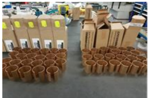
Figure 2 - Packaging on the left with new style bar coding containing bushing with the wide pre-set split line. Packaging on the right without bar coding previously received from Lycoming containing bushing with the narrower split line.
