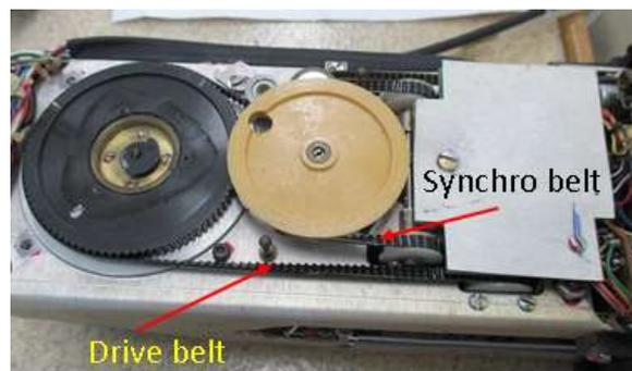
*Figure 3 - Gyro and motor assembly gear*
