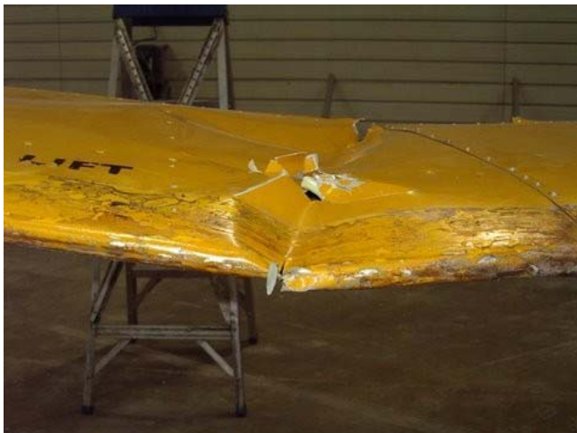
A damaged R/H Horizontal Stabilizer
