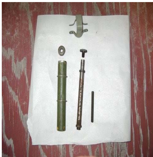
A disassembled R/H Elevator Trim Actuator Assembly
